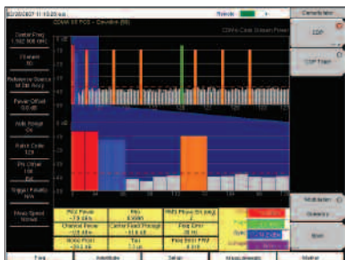
CDMA Code Domain Power measurement display
