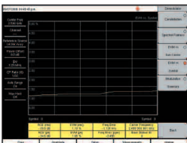
The EVM vs. Symbol displays the EVM (rms) values vs. OFDM Symbols.
