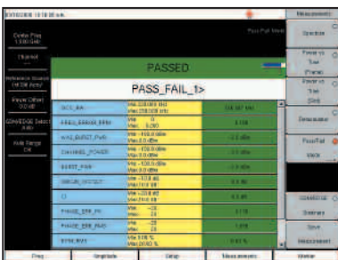
Using Master Software Tools, custom GSM/GPRS/EDGE Pass/Fail test sets can be created and uploaded to the Spectrum Master.
