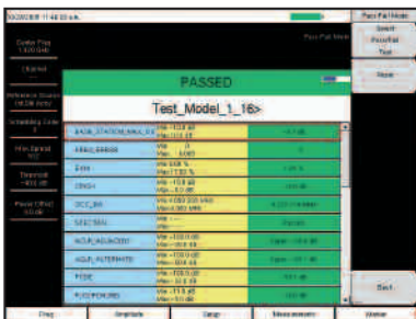
The Spectrum Master offers a clear Pass/Fail display for quick evaluation of a Node B base station.
